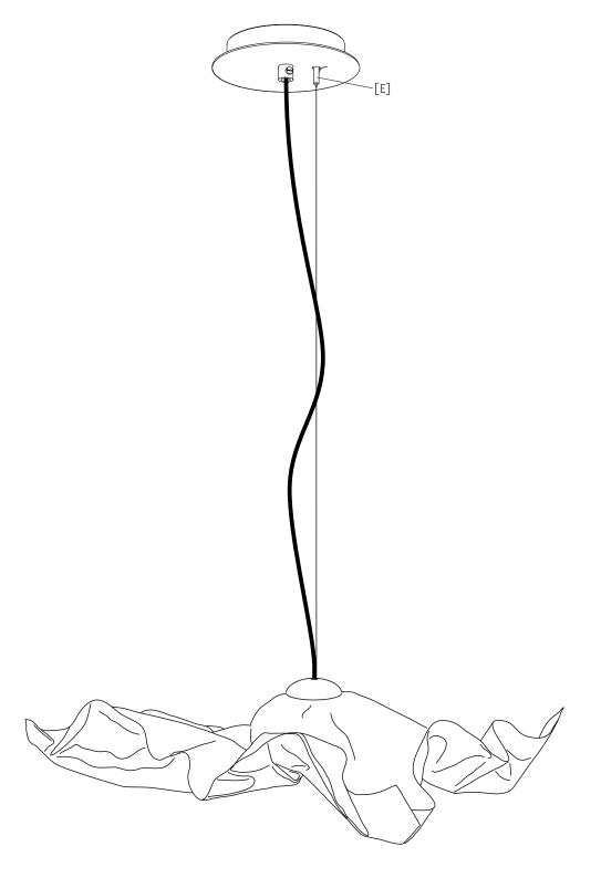
Pass the wire rope through the wire rope holder [E].
