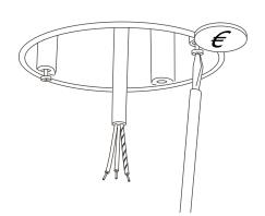
To set the correct distance between the screws on the flush-mounted box, it is best to use a  $1 \in \text{piece}$  as an orientation dimension.
