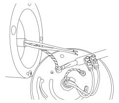
Connect the protective conductor to the Ground connection on the rotary plate.
