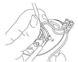
Connect the protective conductor to the Ground connection on the rotary plate.
