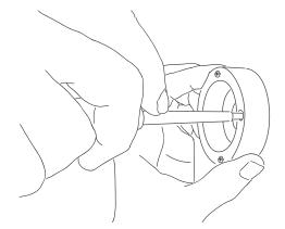
Then fix the enclosed surface box with adequate material (dowels, screws). When drilling, make sure that no cables are damaged.
