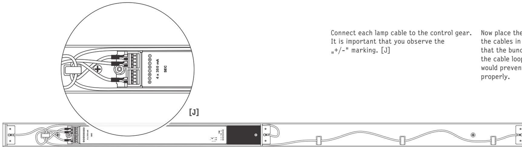
Connect each lamp cable to the control gear. It is important that you observe the „+/-“ marking. [J]
