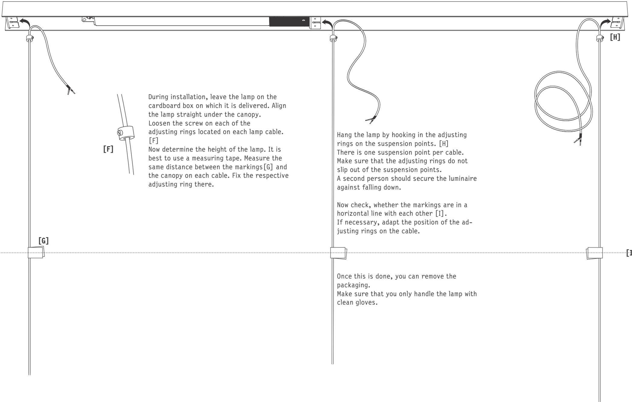
During installation, leave the lamp on the cardboard box on which it is delivered. Align the lamp straight under the canopy. Loosen the screw on each of the adjusting rings located on each lamp cable. [F]
