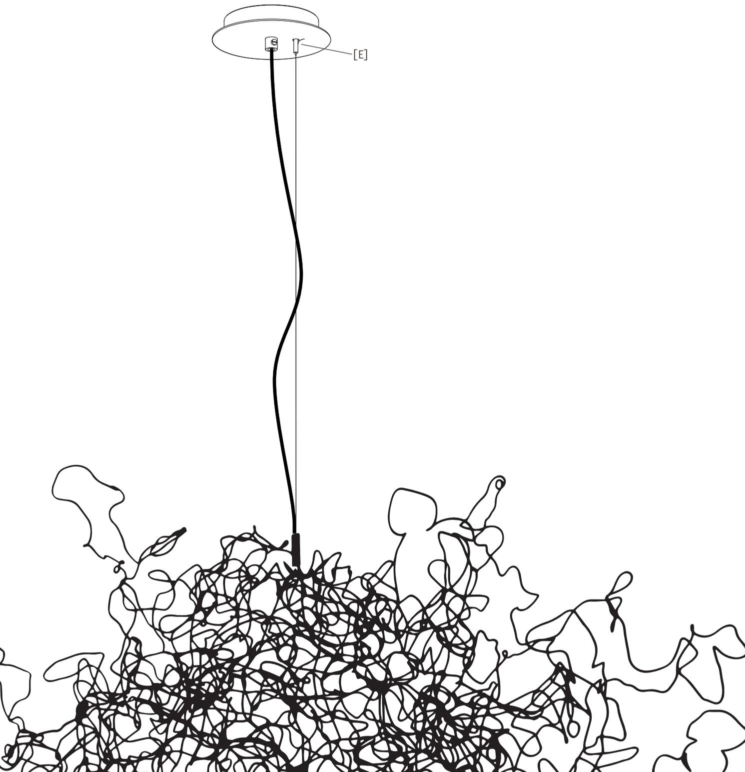
Pass the wire rope through the wire rope holder [E].
