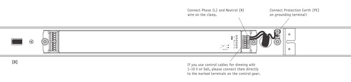
Make sure that the stripped wires are firmly seated in the terminals!
